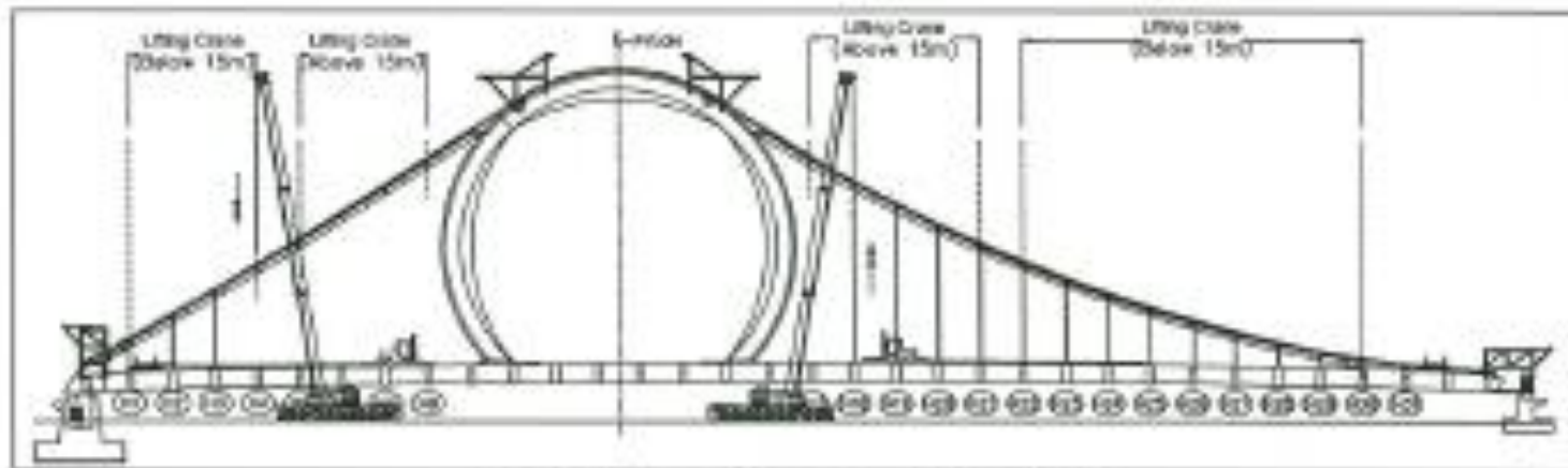
Installation of hanger cable in Br 8
